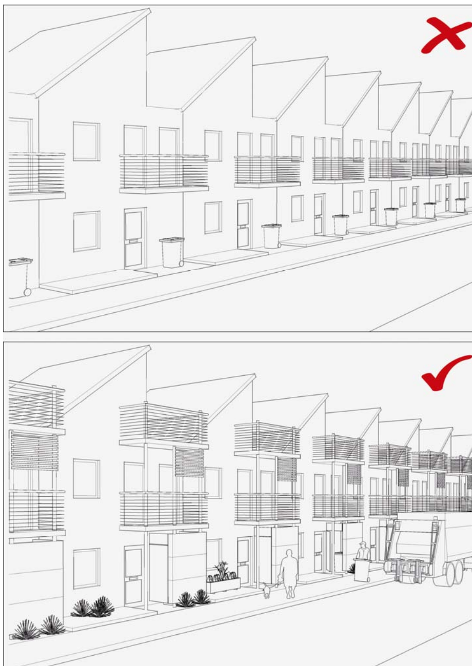
Diagram 6.2 – an example of how dwellings can be designed with enclosed bin storage at the front of the property so that bins are not visible on the street
